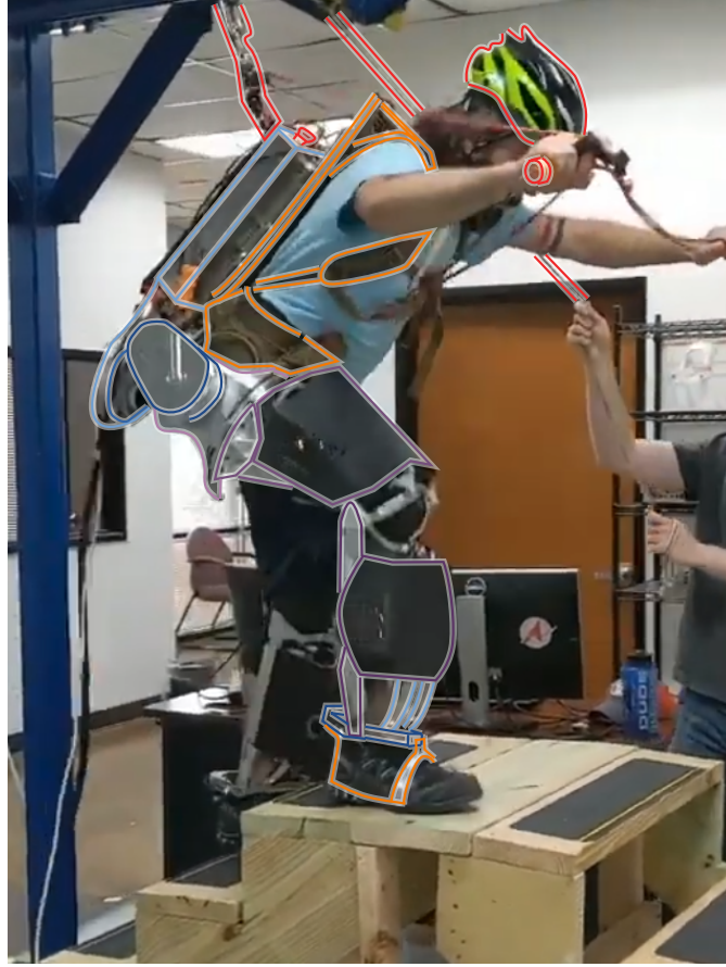
Figure 5. The Appronik Sagittarius Exoskeleton used in this paper. The operator can climb stairs with the exoskeleton, even when it is not amplifying forces, due to the backdrivable torque-controlled actuators (gravity compensation and strength amplification are both active in the pictured movement). Coloring segregates rigid exoskeleton parts for the right leg (blue-through-purple), human interfaces (orange) and the safety features (red).
